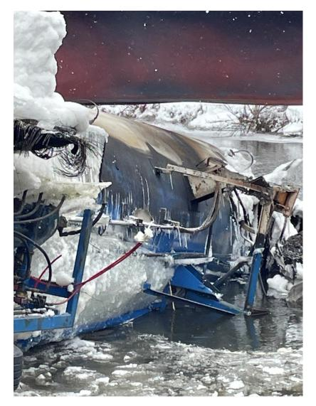
Recovery was a slow process as we still had an active leak and believed to have 800 gals liquid LP in the bottom of the tank. As the Tanker came out of the water we would stop and inspect the tanker's condition.
