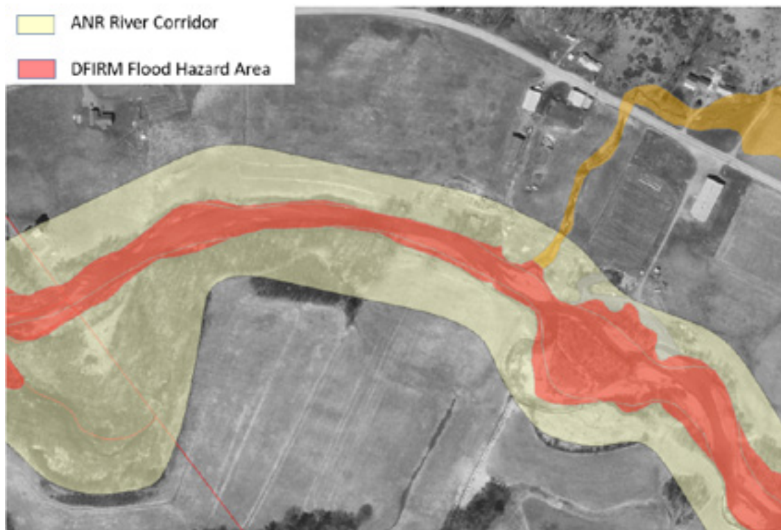
Figure 14: Browns River in Underhill demonstrates the true vulnerability (i.e. River Corridor area) versus the FEMA-mapped vulnerability (DFIRM Flood Hazard Area)
